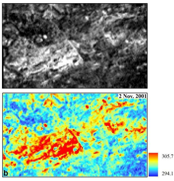
A greyscale and colour-coded thermal temperature image of a coal mine under fire in Dhanbad, India. The brighter the pixel in the temperature image, the higher its temperature will be. The pixels shown as bright white in the centre of the greyscale image above have the highest temperature (305.7  $^{\circ}$ K).
